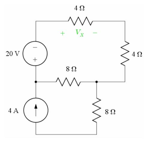
Use superposition to determine the voltage  $V_X$ .
