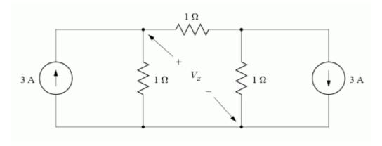
Determine all of the mesh currents in the circuit.
